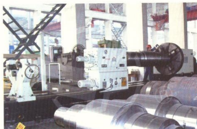
CK61200DX6000数控卧式车床 CK61200DX6000 numerical control horizontal lathe
